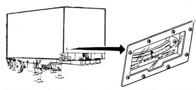
NOTE: Ensure all tires are on the ground and landing jacks are not raised after van is level.
